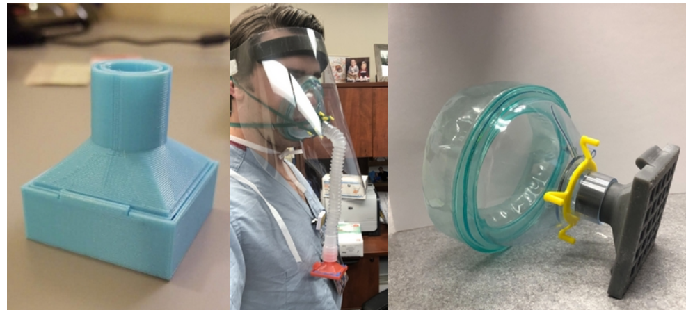
Figure 5 Coupler Prototype and Respirator Design
