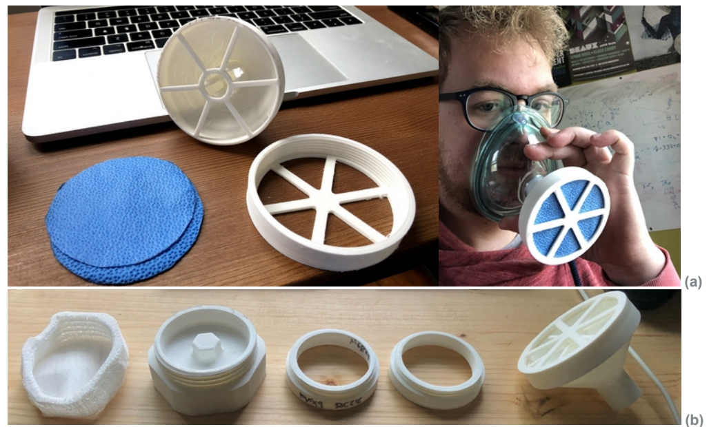
Figure 6 Progression of Threaded Couplings
