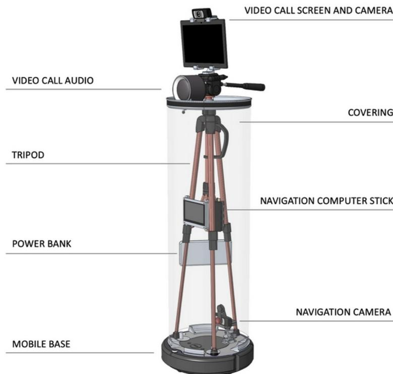
Figure 5. The LHF Connect teleoperated robot.
