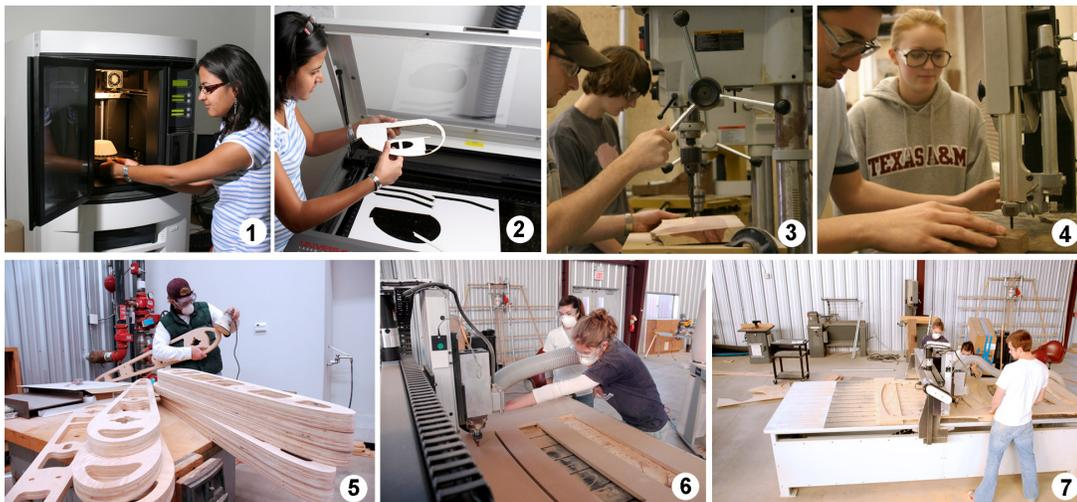
*Figure 4. The College of Architecture Fabrication Facilities: (1) FDM rapid prototyping machine, (2) Laser cutter, (3) (4) Woodshop, (5) (6) (7) CNC milling machine.*
